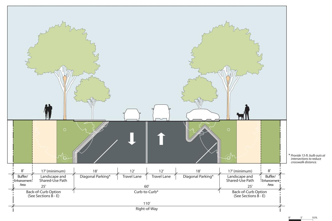
2 Lane Commercial Collector with Diagonal Parking City of Dripping Springs - Transportation Master Plan
